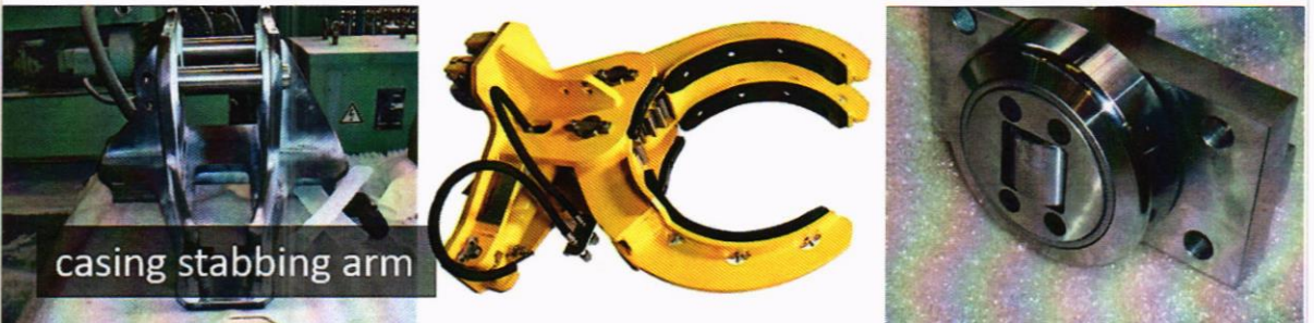
casing tong positioning arms
